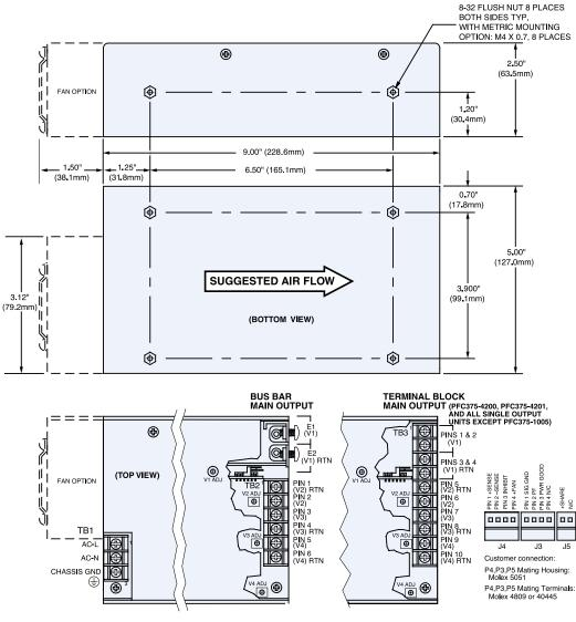
INPUT & OUTPUT CONNECTIONS: 6-32 SCREW TERMINAL ON 0.375" (9.5mm) CENTERS BUS BAR MAIN OUTPUT, E1 & E2, 10-32 SCREW TERMINAL
