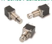
The single or double pole 641-Series represent the most compact offerings of our pushbutton switch line. Rugged metal construction, self cleaning contacts and stiff actuation force (3-3 1/2 lbs. typical) have made these switches ideal for most "foot pedal" type applications. These alternate action switches fit a standard .500" mounting hole, have termination options including solder lug, wire lead and PC, and are popular within the Music Industry and Audio-visual Markets.
