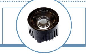
These water-clear polycarbonate lenses with black holders are specifically designed to mate with Optek's 6x6mm power surface mount LEDs (OVSxxxCR4 Series) to provide a more narrow beam angle. Lenses are available in both 15° and 23° viewing angles. The lenses and holders sit firmly over the LED component and is easily attached to the PCB/MCPCB with adhesive.
