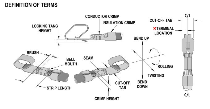
★ Terminal is to be centrally located between the two (2) cut-off edges, within +/- 0.13mm (+/-.005").
