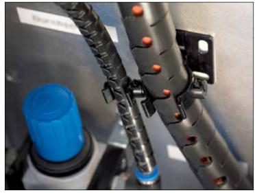
For example: The protection and affixing of cables in a wiring cabinet with Helawrap sleeving.
