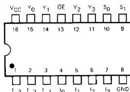
Note: Pin 1 is marked for orientation
