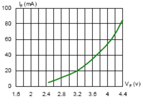
Fig.1 Forward Current vs. Forward Voltage
