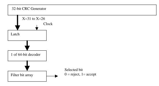
If address Y is found to hash to the value 32 (20H), then FB32 (ref. 4.1.2) in MAR2 should be initialized to 1". This will cause the AX88796B to accept any multicast packet with the address Y. Although the hashing algorithm does not guarantee perfect filtering of multicast address, it will perfectly filter up to 64 logical address filters if these addresses are chosen to map into unique locations in the multicast filter.
