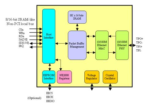
Fig - 1 AX88796B Block Diagram
