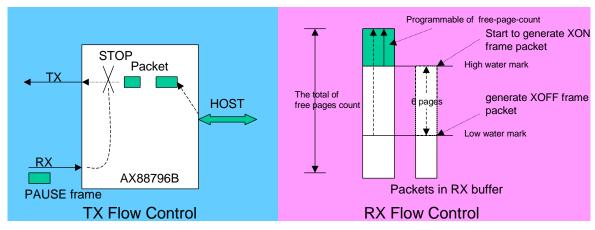
Fig - 6 TX / RX Flow control
