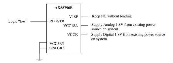
Note: If user connects the VCC3R3 to 3.3V VCC and wants to disable the internal voltage regulator of AX88796B, the REGSTB bit of PMR register should be set to 1 to set the regulator in standby mode to reduce the leakage current.
