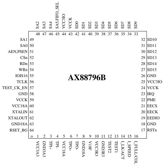
Fig - 2 AX88796B Pin Out Diagram
