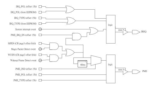
Fig - 8 PME and IRQ signal generation
