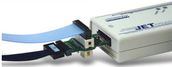
FIGURE 39 The JTAG-ETM splitter board attached to the JTAGjet-Trace emulator. Connected to it are a 20-pin ARM JTAG cable and an ETM Mictor cable (lower). A receptacle for an additional 14-pin TMS320 DSP JTAG cable is located at the bottom of the board.
