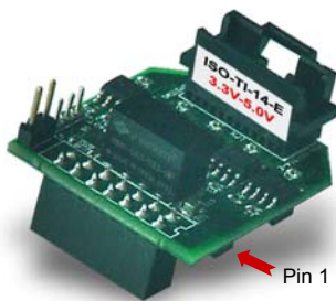
FIGURE 26 The isolation probe for TI-14 JTAG with auxiliary power input ADA-ISO-TI14-E probe with an auxiliary power input.
