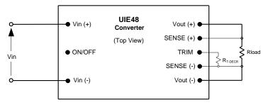
Trimming/sensing beyond 110% of the rated output voltage is not an acceptable design practice, as this condition could cause unwanted triggering of the output overvoltage protection (OVP) circuit. The designer should ensure that the difference between the voltages across the converter's output pins and its sense pins does not exceed 10% of  $V_{OUT}(NOM)$ , or:
