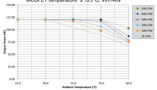
Fig. 4: Power derating vs. ambient air temperature and airflow rates for UIE48T10120 converter w/o baseplate mounted vertically with air flowing from pin 3 to pin 1, MOSEET temperature < 125°C Vin=24U
