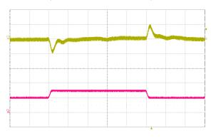
Fig. 13: Output voltage ripple (50 mV/div.) at full rated load current into a resistive load with Co = 10 μF tantalum + 1 μF ceramic and Vin = 48 V. Time scale: 2 μs/div.
