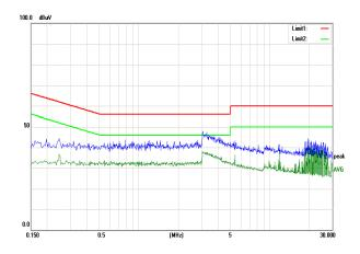
Fig. 20: Vin- Peak Detector EMI waveform
