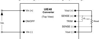
Fig. C: Configuration for increasing output voltage.
