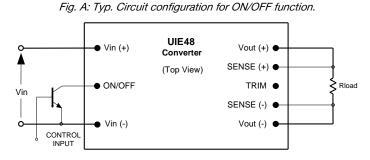
The negative logic version turns on when the ON/OFF pin is at a logic low and turns off when the pin is at logic high. To enable automatic power up of the converter without the need of an external control signal the ON/OFF pin can be hard wired directly to Vin(-) for N and left open for P version.
