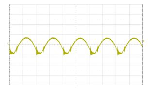
Fig. 15: Input reflected ripple current, ic (1 A/div.), measured at input terminals at full rated load current and Vin = 48 V. Refer to Fig. 14 for test setup. Time scale: 2 µs/div.
