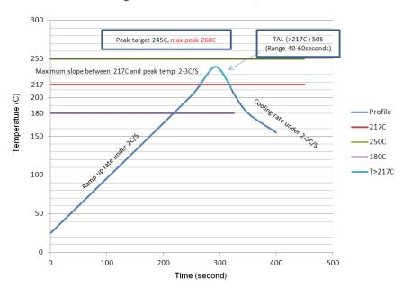
Fig. 21: Lead Free solder reflow profile
