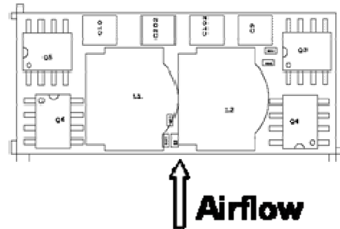
Figure 34. Airflow direction for thermal testing.
