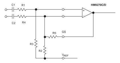
FIGURE 9. DIFFERENTIAL INPUT CONFIGURATION
