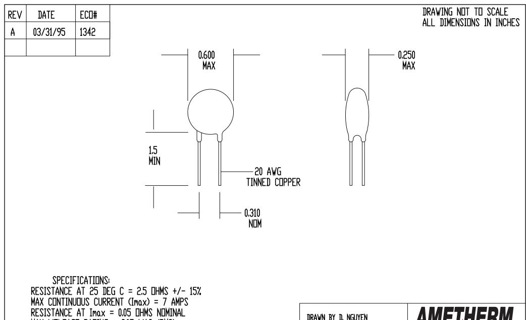
RESISTANCE AT Imax = 0.05 DHMS NDMINAL MAX VOLTAGE RATING = 265 VAC (RMS) MAX SURGE RATING = 27 JOULES ENCAPSULATION = SILICONE RESIN MARKING = DPTIONAL LEADS = RODAN P/N STL-209-20
