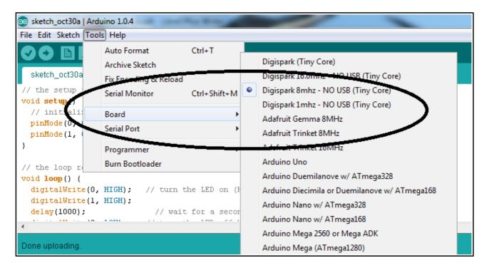
OLIMEXINO-85 is recognized as "Digispark 8mhz - NO USB (Tiny Core)" under "Tools  $\rightarrow$  board"
