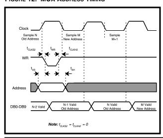
FIGURE 13. ANALOG MUX TIMING
