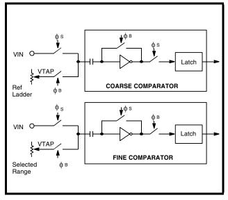
A<sub>IN</sub> Sampling, Ladder Sampling, and Conversion Timing
