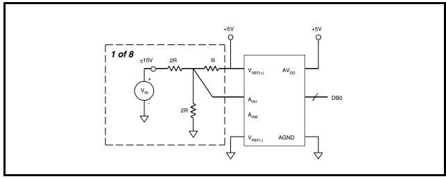
For R = 5k use Beckman Instruments #694-3-R10k resistor array or equivalent.
