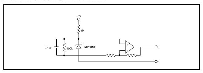
FIGURE 18. ±5V ANALOG INPUT
