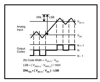
The formulas for Differential Non-Linearity (DNL), Integral Non-Linearity ( $_{\rm IN}$ L) and zero and full scale errors (EZS, EFS) are:
