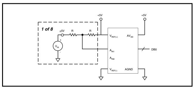
For R = 5k use Beckman Instruments #694-3-R10k resistor array or equivalent.
