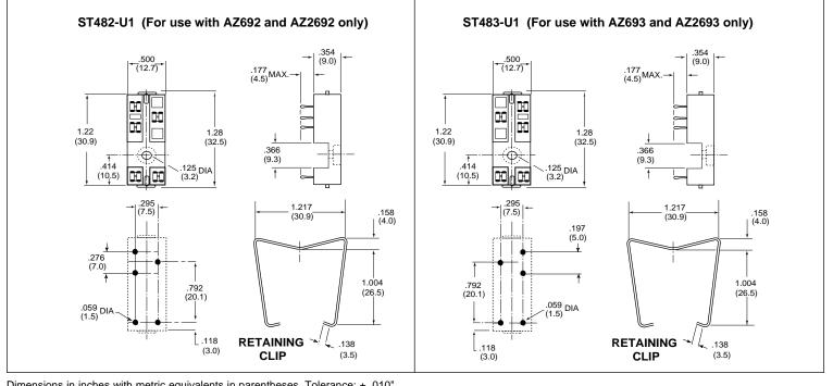
Dimensions in inches with metric equivalents in parentheses. Tolerance:  $\pm$  .010"
