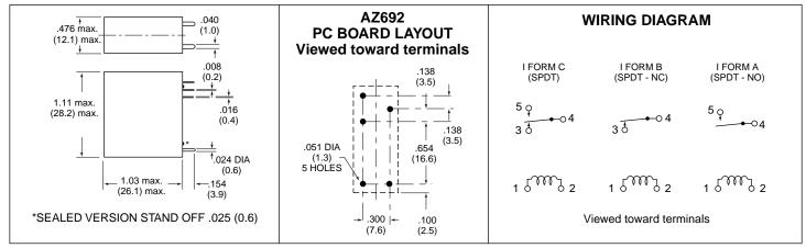
Dimensions in inches with metric equivalents in parentheses. Tolerance: ± .010"
