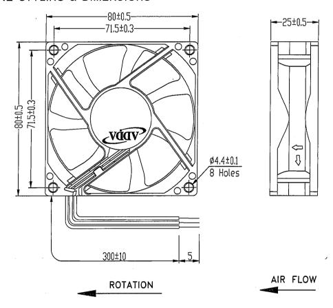
LEAD WIRES: UL 1007, AWG24, L = 300 +/- 10 mm Red = positive; Black = negative.
