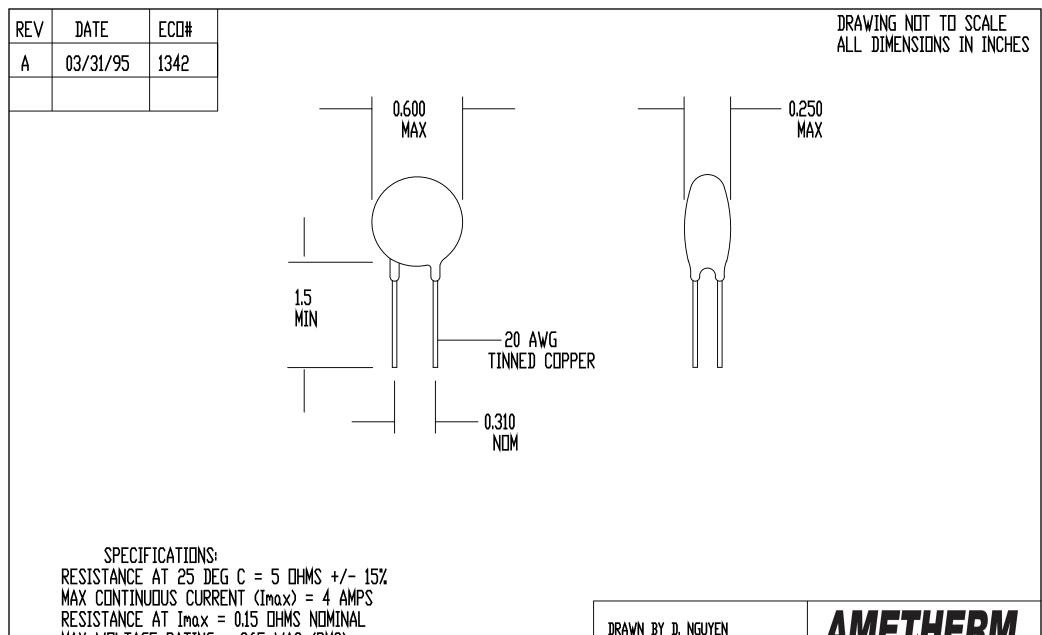
MAX VOLTAGE RATING = 265 VAC (RMS) MAX SURGE RATING = 36 JOULES ENCAPSULATION = SILICONE RESIN MARKING = OPTIONAL LEADS = RODAN P/N STL-209-20
