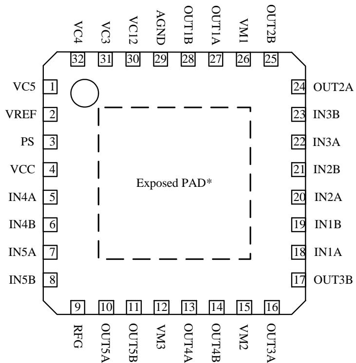
\*The exposed pad must be connected to GND.
