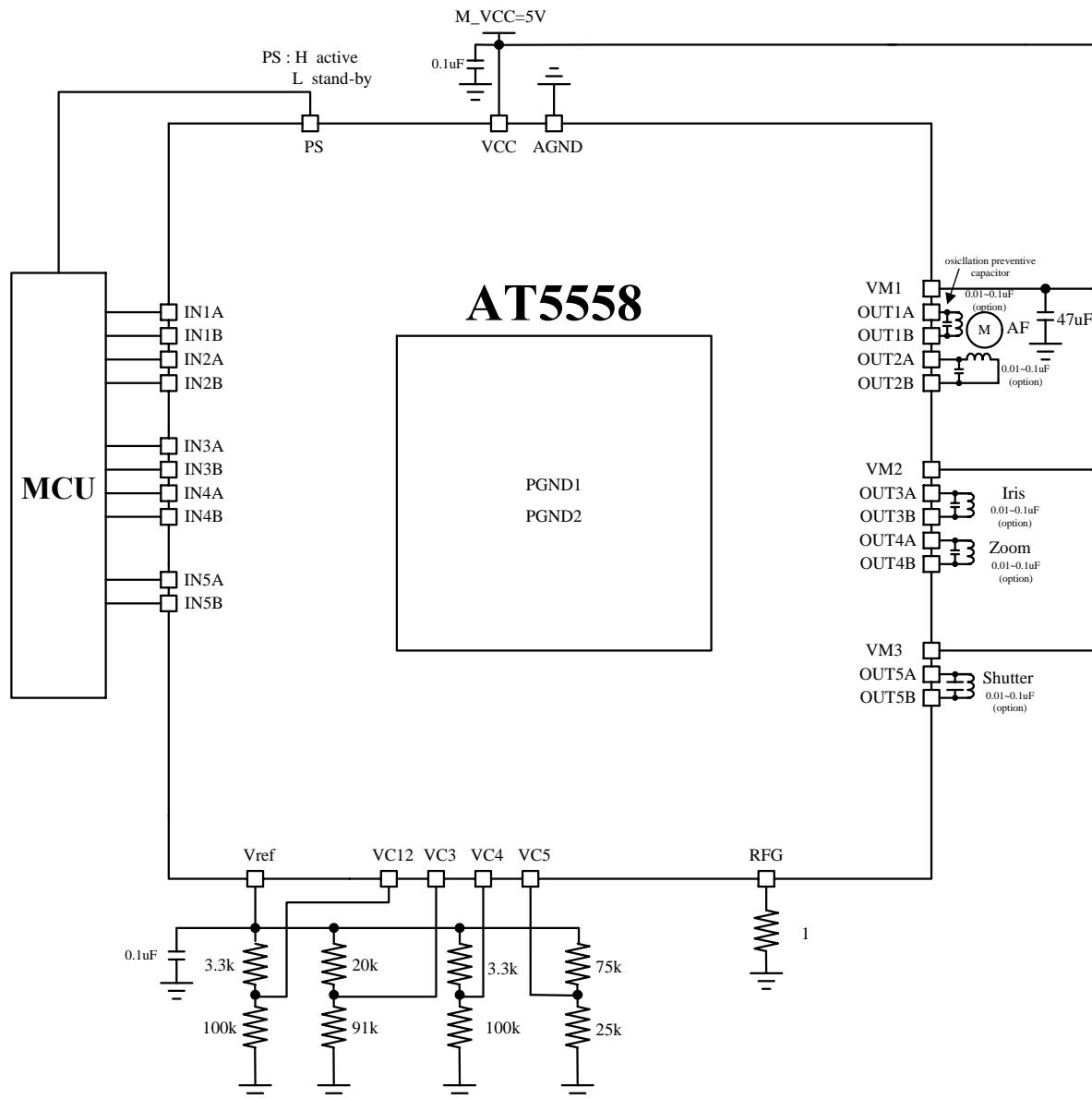
**Constant voltage : CH1&CH2**  $V_{oi} = V_{C12} \times 5 - 0.5 \times R_{ON} \times I_{oi}$ ,  $i = 1, 2$
