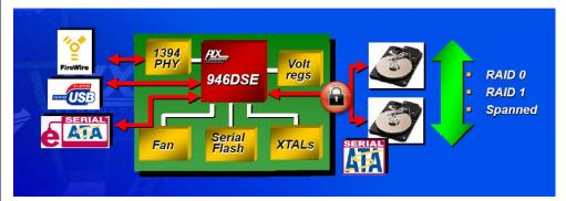
The integrated hardware RAID engine supports a range of RAID modes which deliver either maximum performance (RAID 0), maximum data protection (RAID 1) or maximum capacity (spanning).
