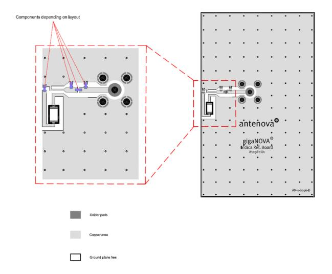
In addition to the matching circuit, a separate DC blocking capacitor will also be required between the radio and the antenna matching circuit.
