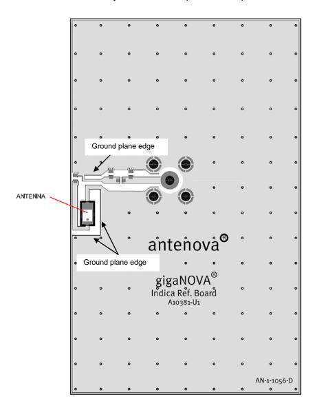
Additional electronic components near the antenna should be at a distance of at least 2 mm away from the ground plane edges. The antenna should also be clear of ground from both the top surface of the antenna and below the antenna.
