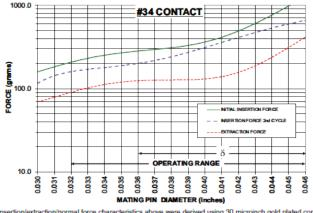
ertion/extraction/normal force cha ristics above were derived using 30 microinch gold plated contact and polished steel gauge pins having a bullet-shaped tip.
