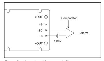
Figure 7 — Secondary side on-state indicator.
