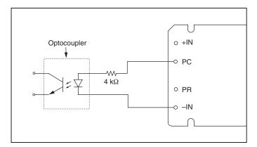
Figure 6 — Isolated on-state indicator.
