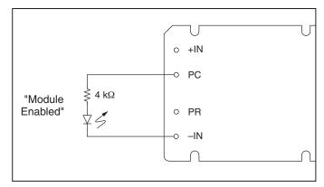
Figure 4 — LED on-state indicator.
