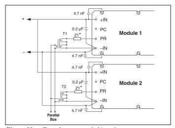
Figure 10 — Transformer-coupled interface.
