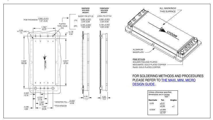
Figure 13 — PCB mounting specifications
