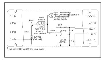
*Figure 3* — *PC/SC module alarm logic.*
