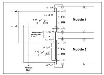
*Figure 9* — *AC coupled single-wire interface.*
