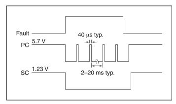
*Figure 5* — *PC/SC module alarm timing.*
