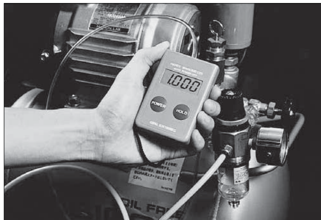
▲コンプレッサの元圧の測定 Measurement of source pressure from a compressor.
