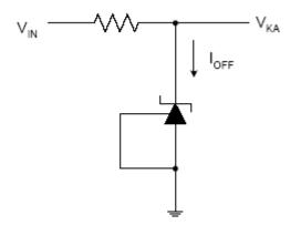
Test Circuit 6 for IOFF
