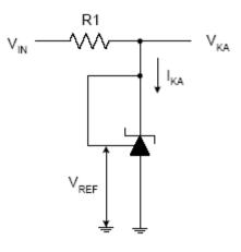
Test Circuit 4 for  $V_{KA} = V_{REF}$
