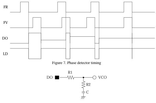
Figure 8. Passive filter
