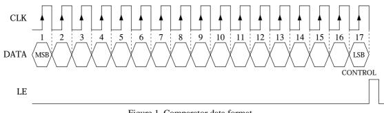
Figure 1. Comparator data format
