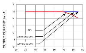
AMBIENT TEMPERATURE,  $T_A$   $^{\circ}C$  Figure 21. Derating Output Current versus Local Ambient Temperature and Airflow (Vin = 3.3Vdc, Vo=2.5 Vdc).
