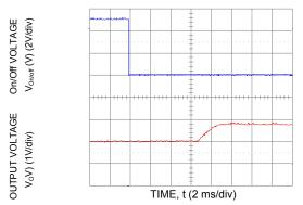
Figure 17 Typical Start-Up using Remote On/off with Prebias (Vin = 3.3Vdc, Vo = 1.8Vdc, Io = 1A, Vbias =1.0 Vdc).
