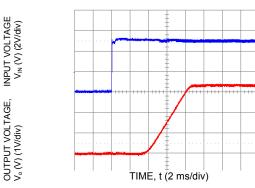
Figure 16. Typical Start-Up with application of Vin with (Vin = 5.0Vdc, Vo = 3.3Vdc, Io = 5A).
