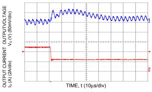
Figure 13. Transient Response to Dynamic Load Change from 100% of 50% full load (Vo = 3.3 Vdc, Cext = 2x150 µF Polymer Capacitors).
