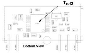
Figure 32. Tref Temperature measurement location.
