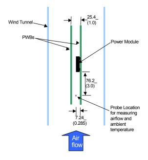
Figure 33. Thermal Test Set-up.
