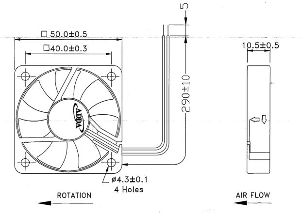
LEAD WIRES: UL 1007, AWG26, L = 290 +/- 10 mm Red = positive; Black = negative.
