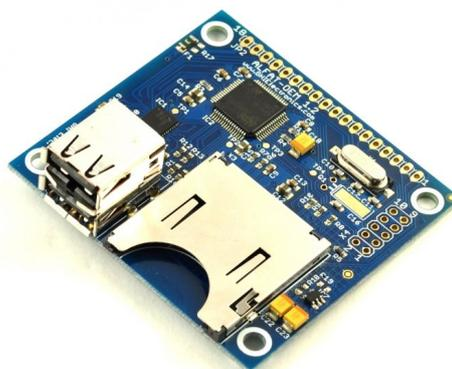
All required signals are exposed through a 1x18 pin-mount. Also, if the desired interface is UART, all signals required are exposed through a secondary 2x5 pin-mount.
