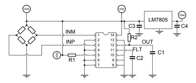
With the use of an external voltage regulator to supply the sensor, the MLX90326 as well as an ADC used for converting the analog output signal, the MLX90326 can be used in a non ratio-metric mode. An example of
