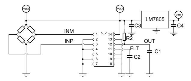
In this application mode the LM7805 generates the supply for the sensor, for the MLX90326 and for an ADC used to convert the analog output signal in a digital value. C1, C2, C3, C4 and R2 are the same as in the non ratio-metric application mode with external temperature sensor.
