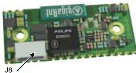
Picture 6: JST 6-pol connector, J8.
