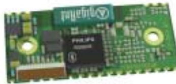
Picture 2: CB-OEMSPA311i-07 OEM Serial Port Adapter short range with internal antenna and a flexfilm connector
