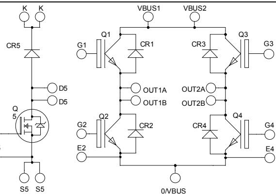
Full bridge top switches : Trench + Field Stop IGBT3
