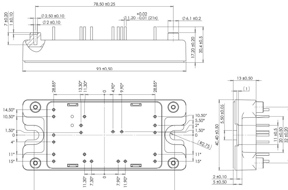
ALL DIMENSIONS MARKED " \* " ARE TOLERENCED AS  $\phi \pm 1$
