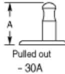
Cheat Interlock Pulled out - 30A
