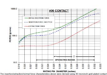
The insertion extraction information of characteristics above were derived using 30 micromoting gold pated contact and polished steel gauge pins having a bullet-shaped tip. The curves represent twoical average values: they are best used to compare the differences between similar size
