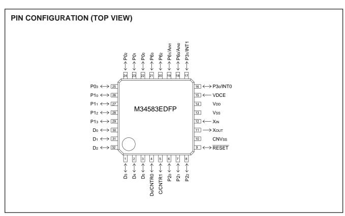
Fig. 69 Pin configuration of built-in PROM version
