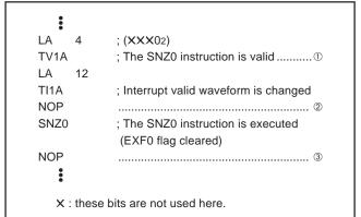
Fig. 61 External 0 interrupt program example-3
