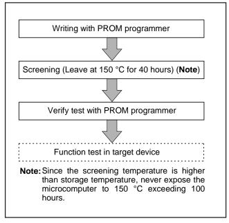
Fig. 71 Flow of writing and test of the product shipped in blank
