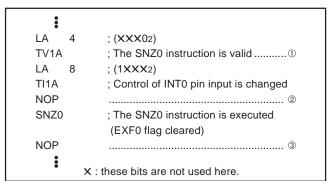
Fig. 59 External 0 interrupt program example-1
