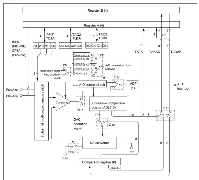
Notes 1: This switch is turned ON only when A-D converter is operating and generates the comparison voltage.
