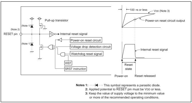
Fig. 42 Structure of reset pin and its peripherals,, and power-on reset operation
