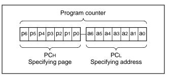
Fig. 7 Program counter (PC) structure
