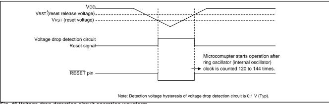
Fig. 46 Voltage drop detection circuit operation waveform
