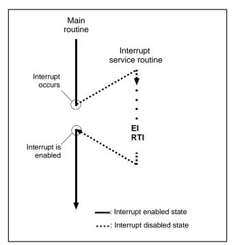
Fig. 13 Program example of interrupt processing
