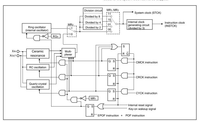
Fig. 51 Clock control circuit structure
