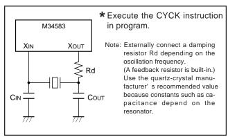
Fig. 56 External quartz-crystal circuit
