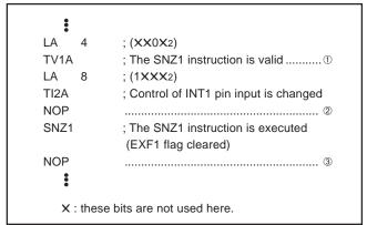
Fig. 21 External 1 interrupt program example-1
