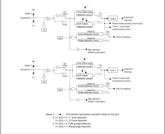
Fig. 17 External interrupt circuit structure
