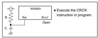
Fig. 55 External RC oscillation circuit
