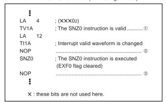
Fig. 20 External 0 interrupt program example-3
