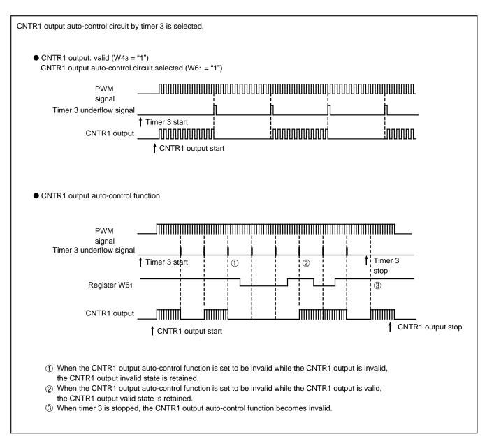
Fig. 30 CNTR1 output auto-control function by timer 3
