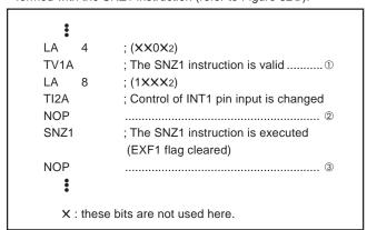
Fig. 62 External 1 interrupt program example-1
