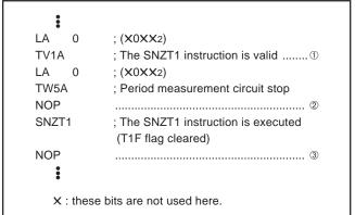
Fig. 28 Period measurement circuit program example
