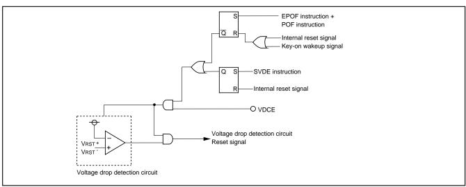
Fig. 45 Voltage drop detection reset circuit
