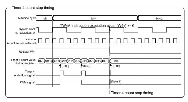
Notes 1: In order to stop timer 4 at CNTR1 output valid (W4 $_3$  = "1"), avoid a timing when timer 4 underflows. If these timings overlap, a hazard may occur in a CNTR1 output waveform.
