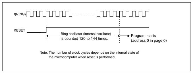
Fig. 40 Reset release timing
