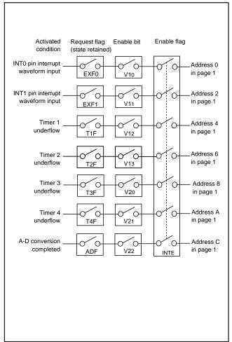
Fig. 15 Interrupt system diagram
