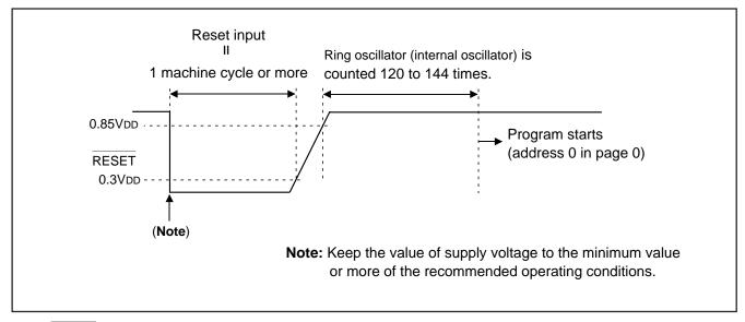
Fig. 41 RESET pin input waveform and reset operation
