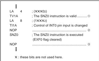
Fig. 18 External 0 interrupt program example-1
