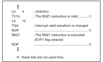
Fig. 23 External 1 interrupt program example-3
