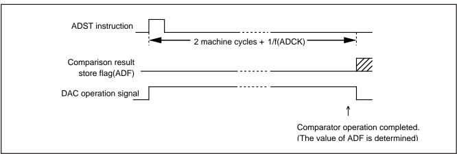
Fig. 38 Comparator operation timing chart
