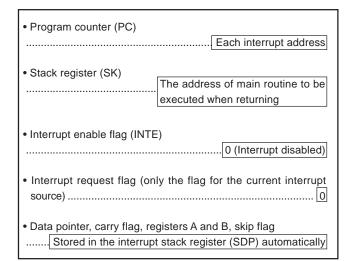
Fig. 14 Internal state when interrupt occurs
