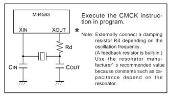
Fig. 54 Ceramic resonator external circuit
