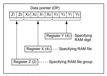
Fig. 8 Data pointer (DP) structure
