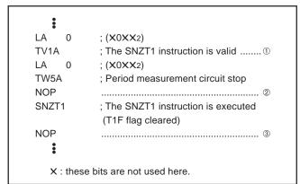
Fig. 27 Period measurement circuit program example
