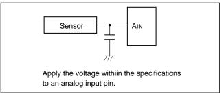
Fig. 66 Analog input external circuit example-1
