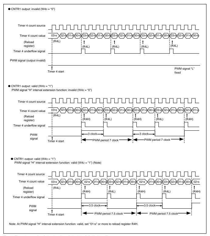
Fig. 29 Timer 4 operation (reload register R4L: "0316", R4H: "0216")
