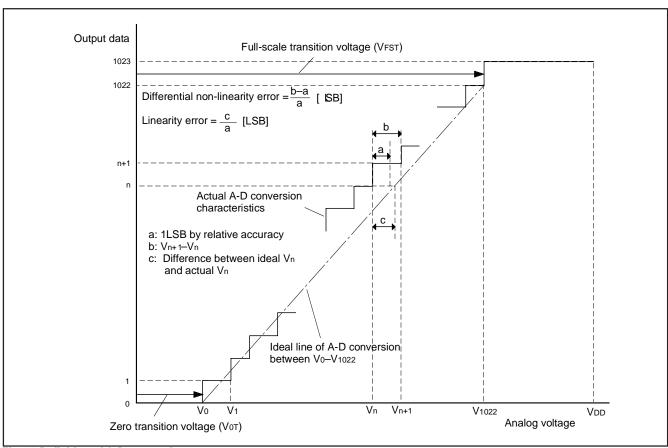
Fig. 39 Definition of A-D conversion accuracy
