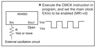
Fig. 57 External clock input circuit
