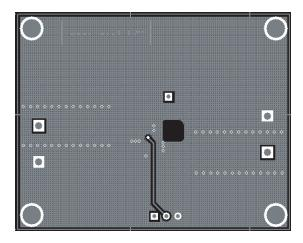
Figure 4: AAT1141 Sample Layout Bottom Side.
