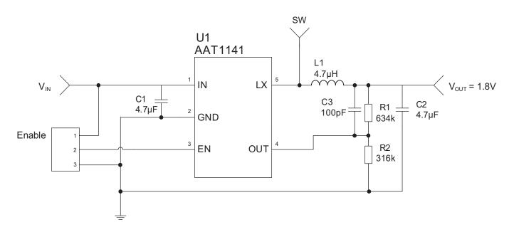
Figure 5: AAT1141 Adjustable Evaluation Board Schematic.
