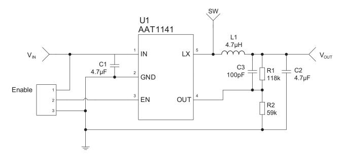
Figure 1: Enhanced Transient Response Schematic.
