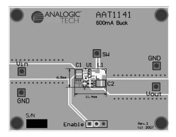
Figure 2: AAT1141 Sample Layout Top Side.
