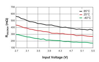
N-Channel R<sub>DS(ON)</sub> vs. Input Voltage
