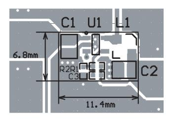
Figure 3: Exploded View of Sample Layout.
