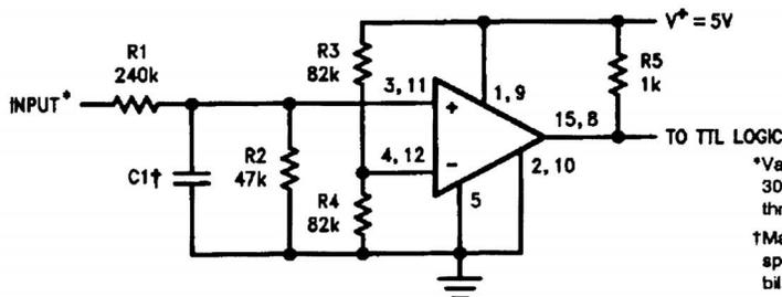
\*Values shown are for a 0V to 30V logic swing and a 15V threshold.
