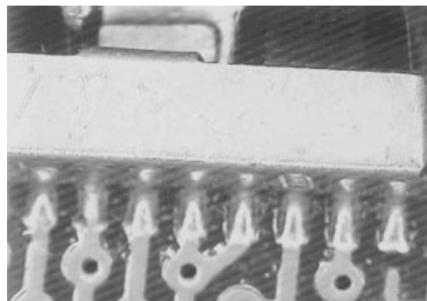
Picture 4. Unit self-aligns after reflow.
