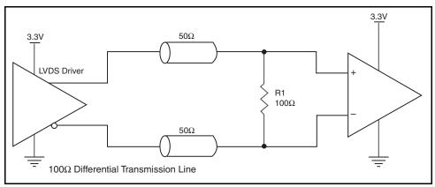
Figure 1. Typical LVDS Driver Termination
