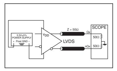
3.3V LVDS Output Load AC Test Circuit
