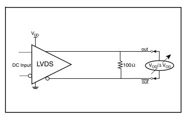
**Differential Output Voltage Setup**
