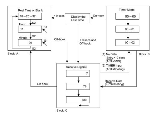
Note: Block A shows the switches S1 and S2 that are used for setting and selecting when RT=VDD (Real time mode). S1 and S2 are disabled when RT= floating (Blank mode).
