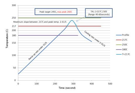
Fig. 21: Lead Free solder reflow profile
