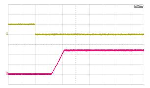
Fig. 11: Output voltage response to load current stepchange(7A – 10.5 A –7 A) at Vin = 48 V. Current slew rate: 0.1 A/μs. Co = 470μF E-cap +1 μF ceramic + 10 μF tantalum. Time scale: 100 μs/div.
