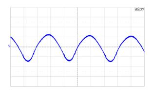
Fig. 16: Input reflected ripple current, i<sub>s</sub> (20 mA/div.), measured through 10 µH at the source at full rated load current and Vin =48 V. Refer to Fig. 14 for test setup. Time scale: 2 µs/div.
