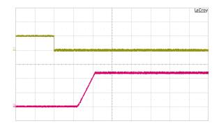
Fig. 12: Output voltage response to load current stepchange(7A – 10.5A – 7A) at Vin = 48 V. Current slew rate: 0.1 A/μs. Co = 4700μF E-cap +1 μF ceramic + 10 μF tantalum. Time scale: 500 μs/div.
