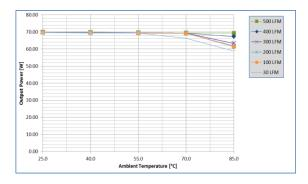
Fig. 6: Power derating vs. ambient air temperature and airflow rates for UIS48T14050 converter with baseplate equipped with .45" finned heatsink mounted vertically with air flowing from pin 3 to pin 1, MOSFET temperature ≤ 125°C, Vin=48V
