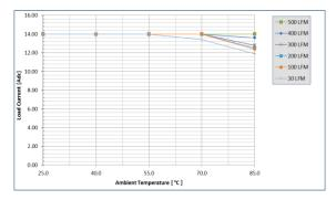
Fig. 5: Available load current vs. ambient air temperature and airflow rates for UIS48T14050 converter with baseplate equipped with .45" finned heatsink mounted vertically with air flowing from pin 3 to pin 1, MOSFET temperature ≤ 125°C, Vin=48V
