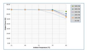
Fig. 4: Power derating vs. ambient air temperature and airflow rates for UIS48T14050 converter w/o baseplate mounted vertically with air flowing from pin 3 to pin 1, MOSFET temperature ≤ 125°C, Vin=24V
