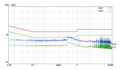
Fig. 20: Vin- Peak Detector EMI waveform
