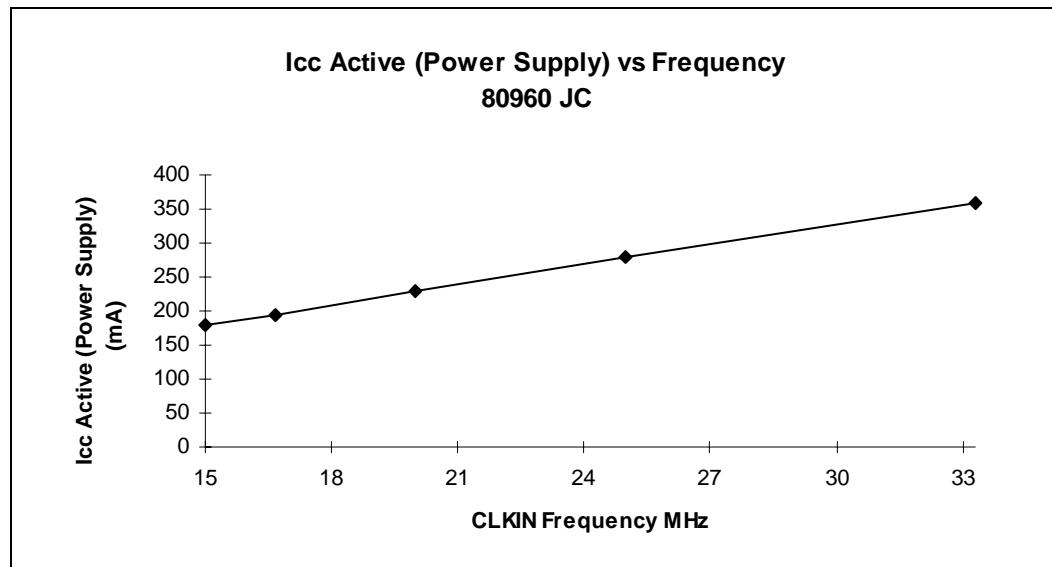
**Figure 22. 80960JC  $I_{CC}$  Active (Thermal) vs. Frequency**
