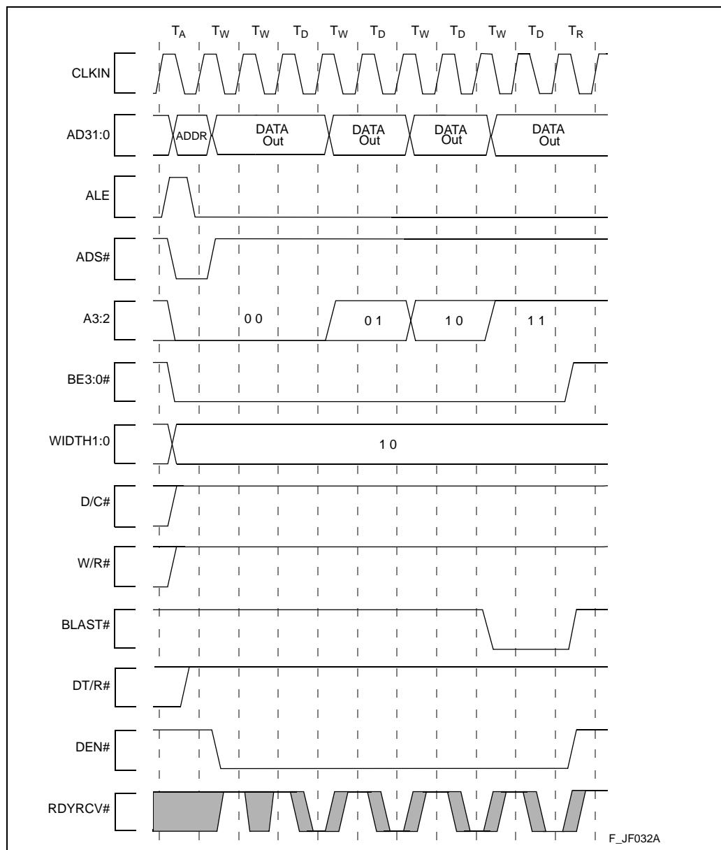
Figure 42. Burst Read and Write Transactions Without Wait States, 8-Bit Bus
