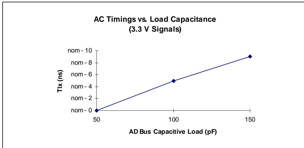
**Note:** The  $T_{LX}$  Derating curve applies only when an imbalance in the capacitive load occurs between the AD bus and ALE. The  $T_{LX}$  derating is based on a 50 pF load on ALE. The derating applies to ALE and ALE#.
