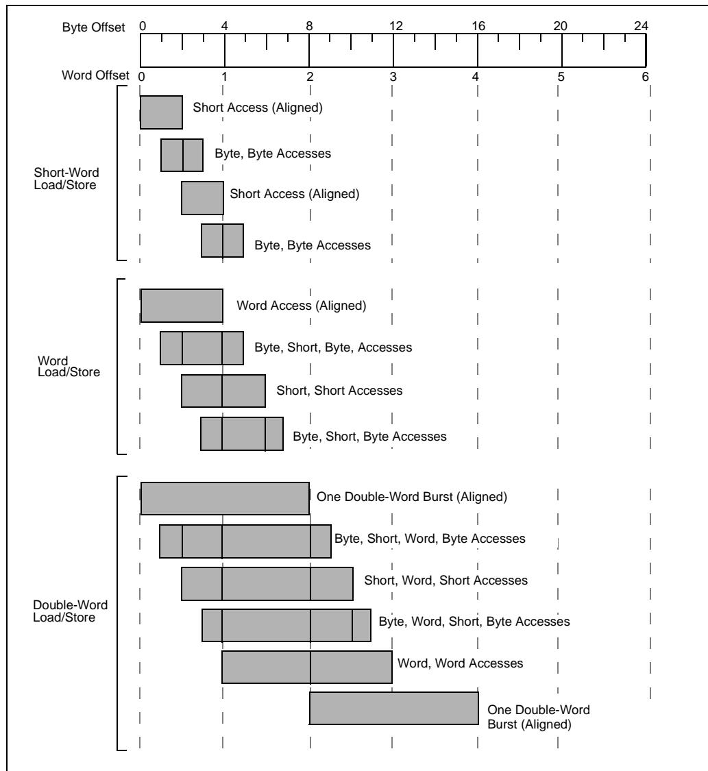
**Figure 51. Summary of Aligned and Unaligned Accesses (32-Bit Bus) (Continued)**
