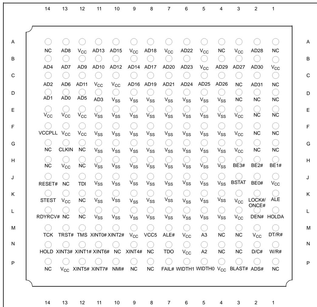
Table 15. 196-Ball MPBGA Pinout — In Signal Order (Sheet 1 of 2)
