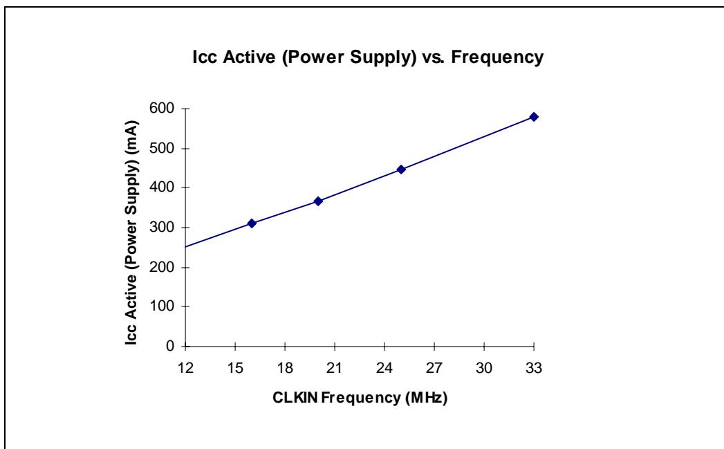
Figure 20. 80960JD  $I_{CC}$  Active (Thermal) vs. Frequency
