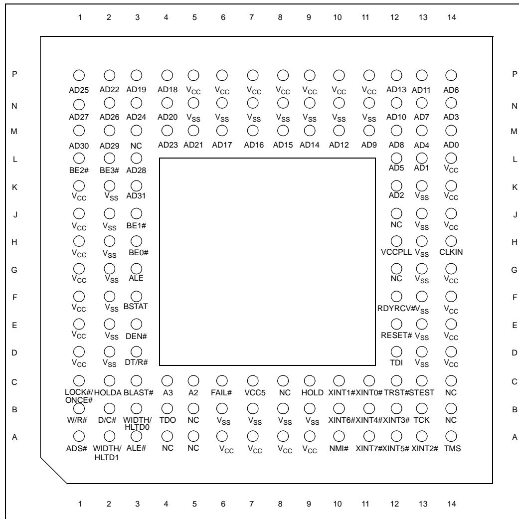
**Table 11. 132-Lead PGA Pinout — In Signal Order**
