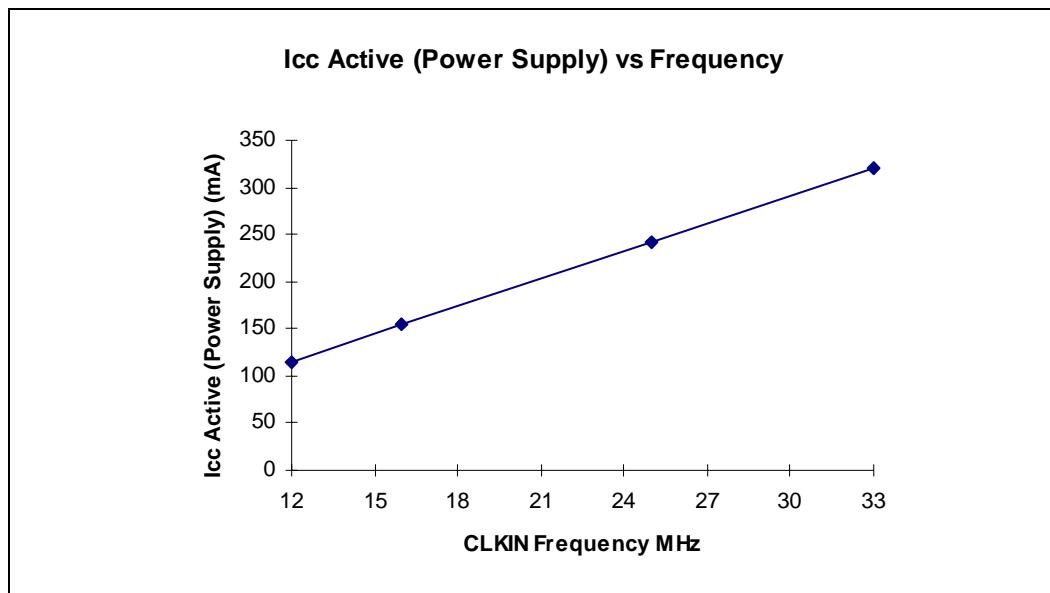
Figure 18. 80960JA/JF  $I_{CC}$  Active (Thermal) vs. Frequency
