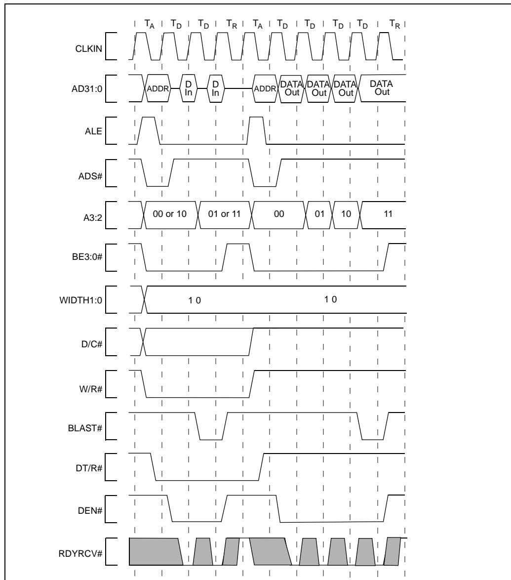
**Figure 41. Burst Write Transactions With 2,1,1,1 Wait States, 32-Bit Bus**
