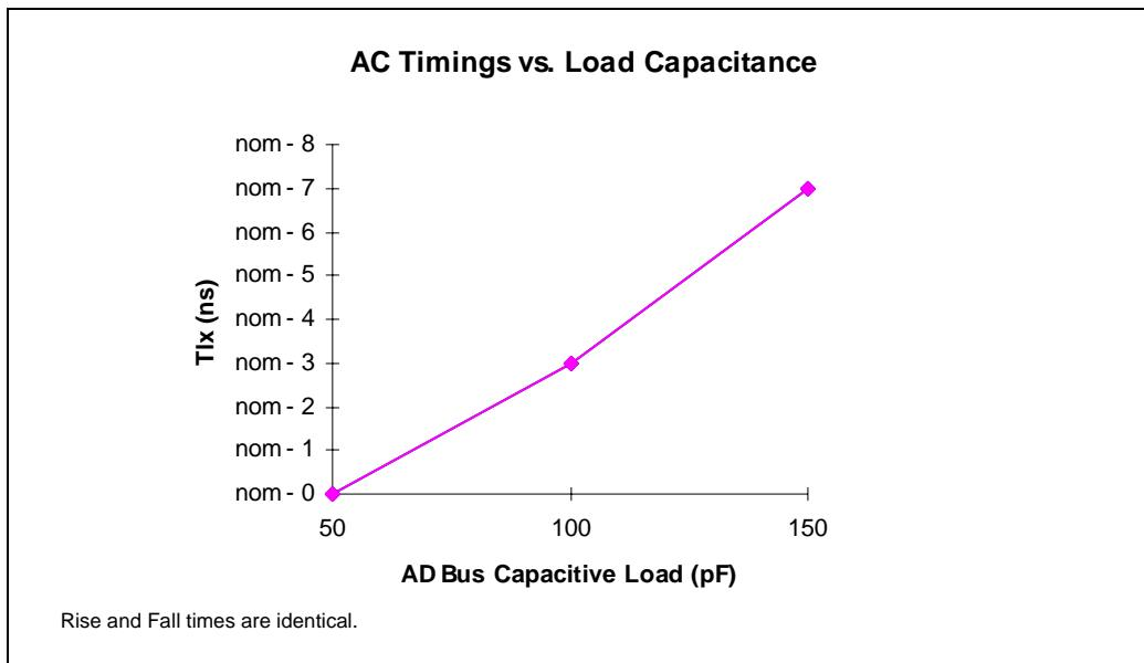
**Note:** The  $T_{LX}$  Derating curve applies only when an imbalance in the capacitive load occurs between the AD bus and ALE. The  $T_{LX}$  derating is based on a 50 pF load on ALE. The derating applies to ALE and ALE#.
