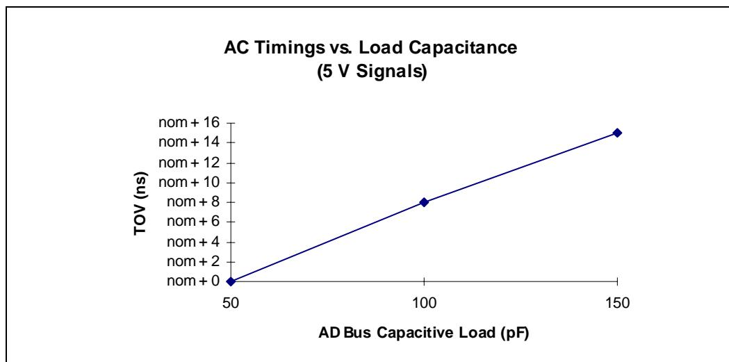
Figure 13. Output Delay or Hold vs. Load Capacitance – 80960JA/JF/JD
