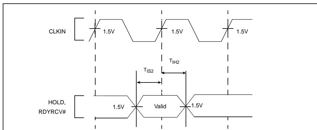
**Figure 30.  $T_{IS3}$  and  $T_{IH3}$  Input Setup and Hold Waveform**
