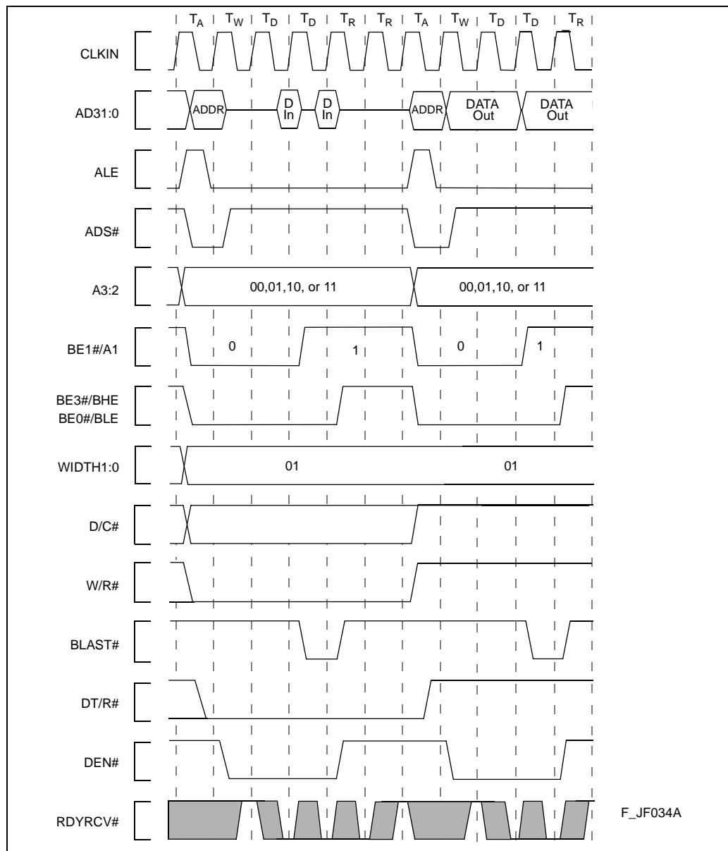
**Figure 44. Double Word Read Bus Request, Misaligned One Byte From Quad Word Boundary, 32-Bit Bus, Little Endian**
