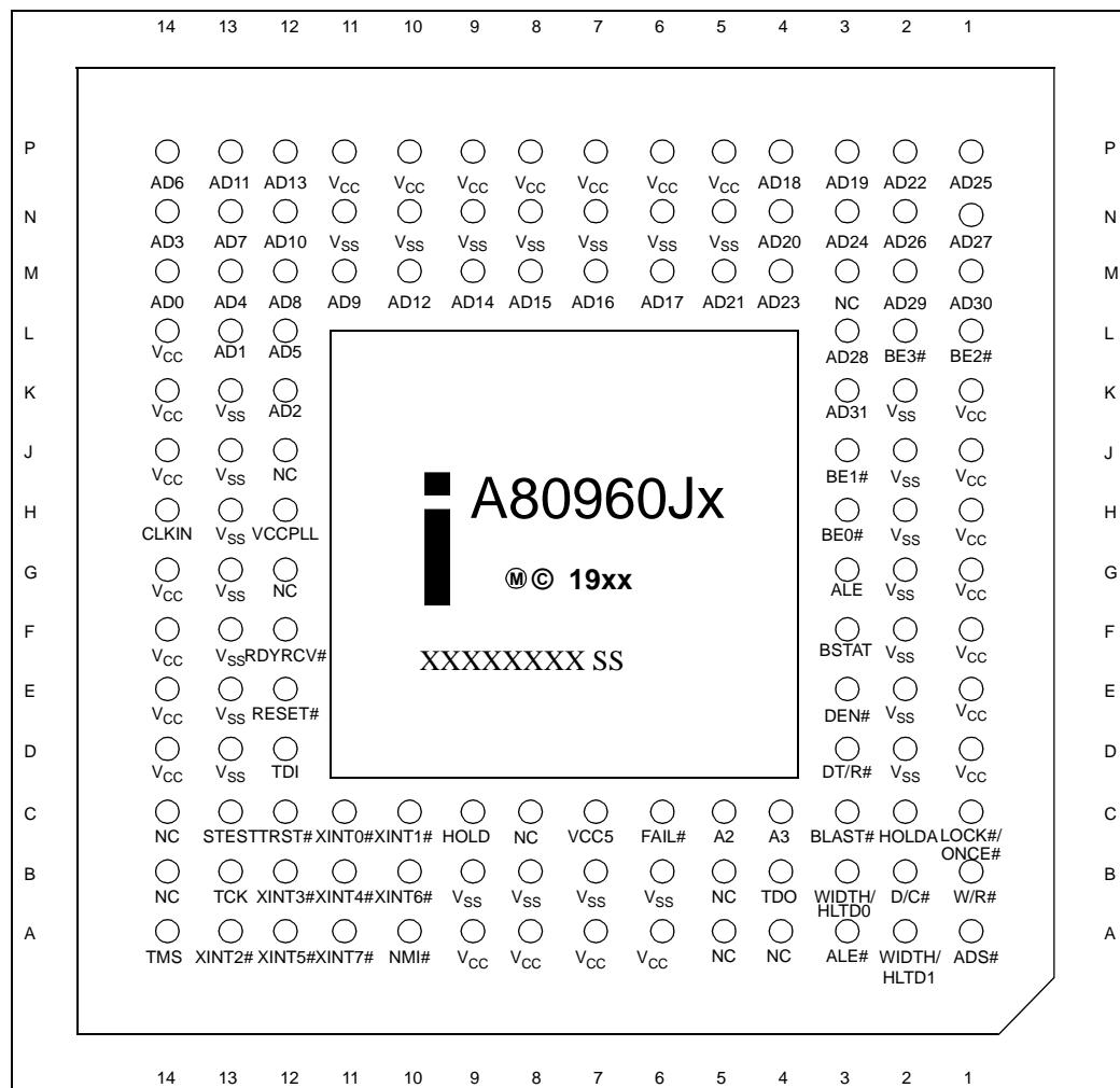
Figure 4. 132-Lead Pin Grid Array Bottom View - Pins Facing Up
