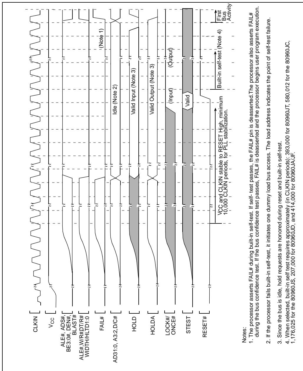
**Figure 47. Warm Reset Waveform**
