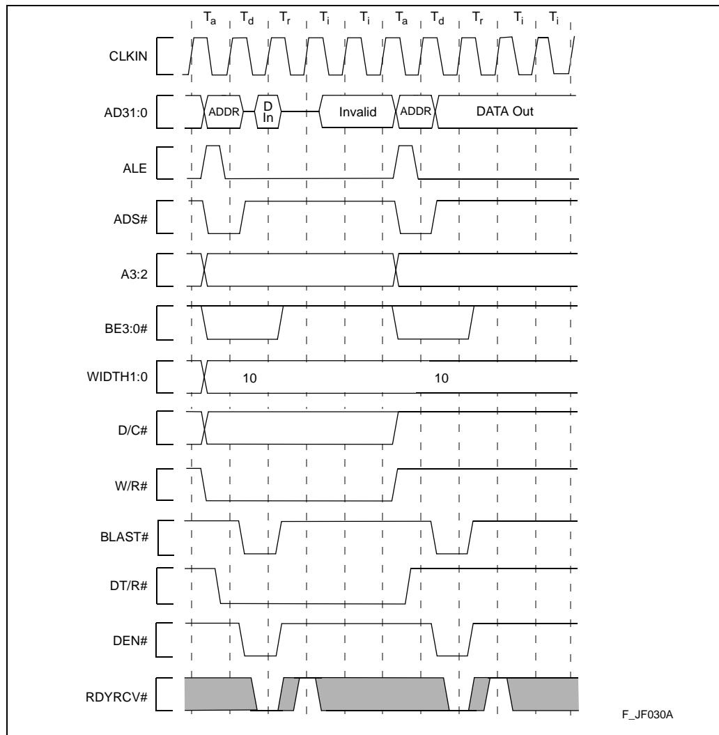
Figure 40. Burst Read and Write Transactions Without Wait States, 32-Bit Bus
