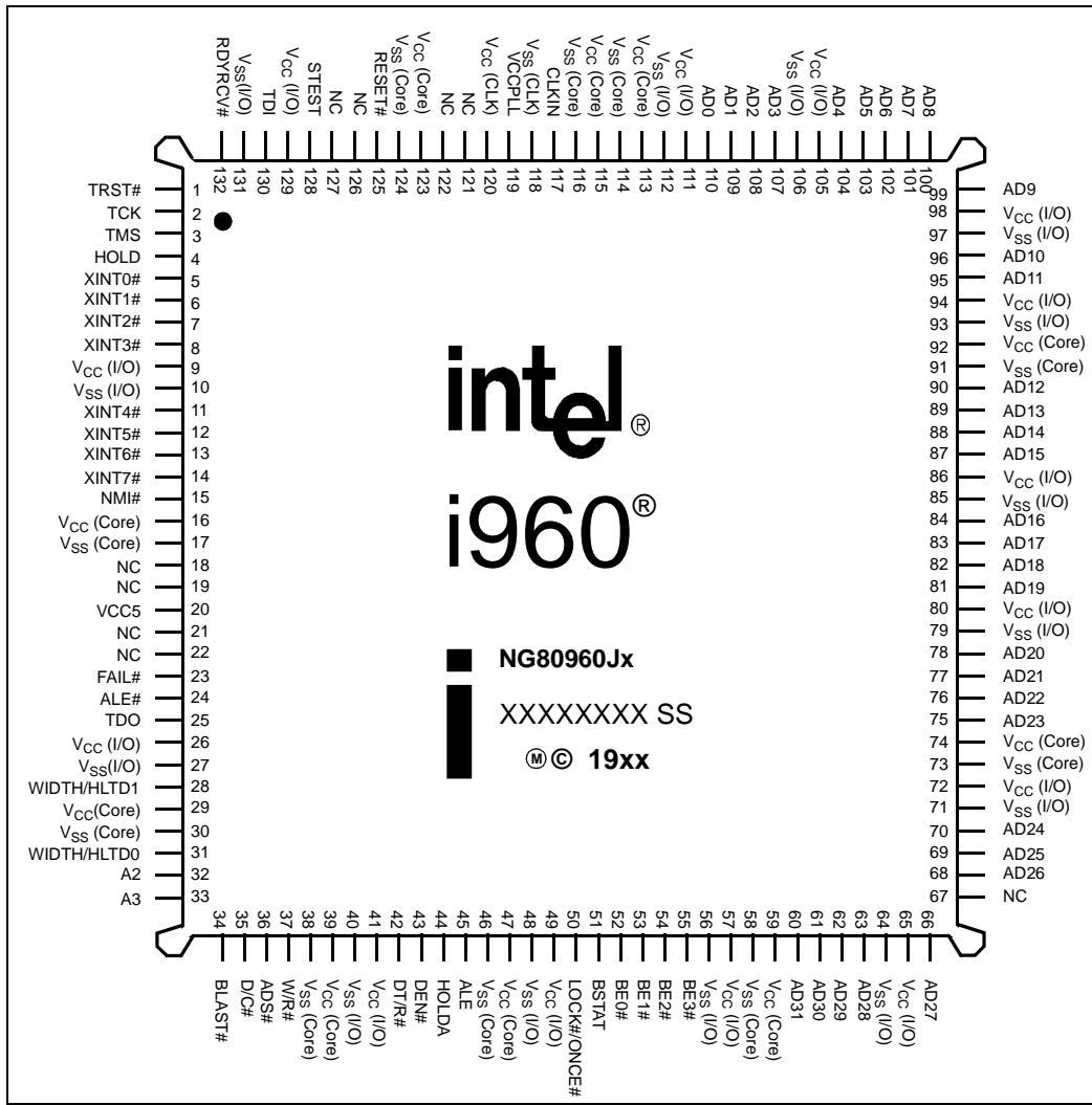
**Table 13. 132-Lead PQFP Pinout — In Signal Order**
