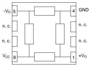
Figure 1: internal and external connections (TDFN, Chip)
