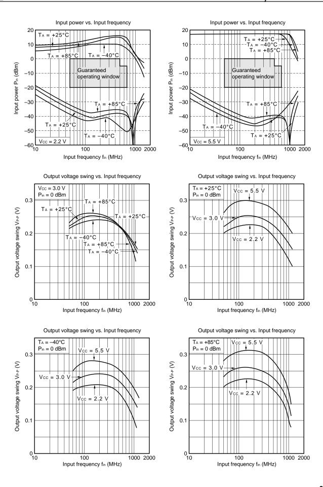
Divide by 4 mode (Guaranteed operating window: Vcc = 2.2 to 5.5 V, TA = -40 to +85°C)
