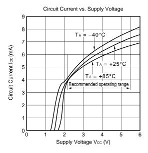
Divide by 2 mode (Guaranteed operating window: Vcc = 2.2 to 5.5 V, TA = -40 to +85°C)
