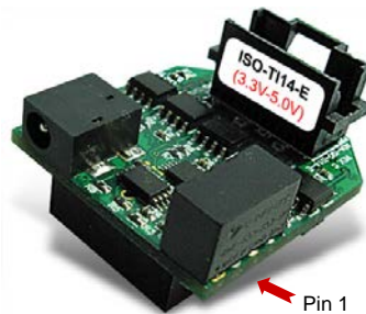
FIGURE 25 The ADA-ISO-TI14-E isolation probe with an auxiliary power input.
