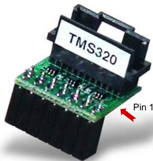
FIGURE 17 The 14-pin JTAGjet probe for OMAP and TMS320 DSP.
