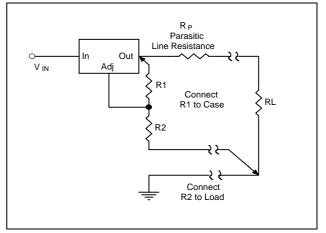
the top of  $R_1$  is internally connected to the output and ground pin can be connected to low side of the load as a negative side sense if, so desired.
