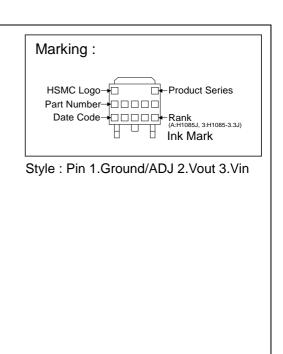
3-Lead TO-252 Plastic Surface Mount Package HSMC Package Code : J
