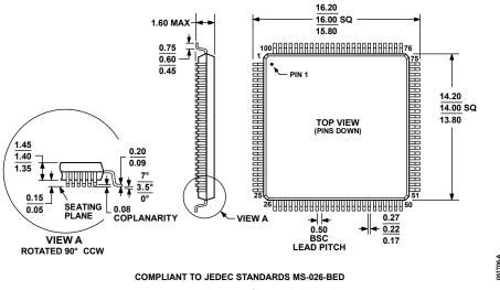
Figure 36. 100-Lead Low Profile Quad Flat Package [LQFP] (ST-100) Dimensions shown in millimeters
