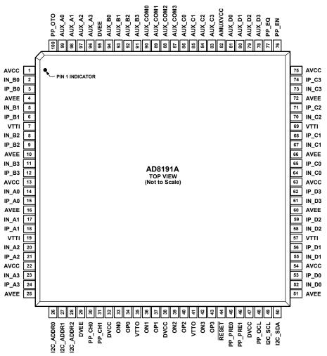
Figure 3. Pin Configuration
