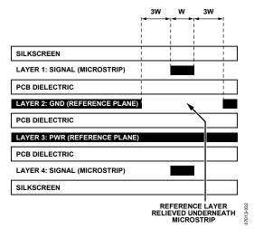
Figure 33. Example Board Stackup
