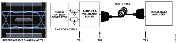
Figure 9. Test Circuit Diagram for Tx Eye Diagrams
