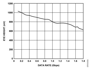
Figure 18. Eye Height vs. Data Rate
