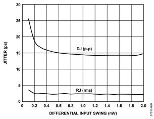
Figure 20. Jitter vs. Differential Input Swing
