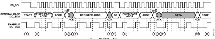
Figure 30. I<sup>2</sup>C Read Diagram
