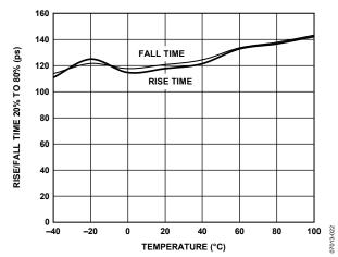
Figure 22. Rise/Fall Time vs. Temperature
