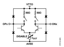
Figure 26. High Speed Output Simplified Schematic
