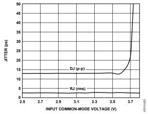
Figure 23. Jitter vs. Input Common-Mode Voltage
