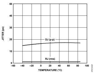
Figure 21. Jitter vs. Temperature
