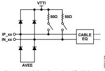
Figure 25. High Speed Input Simplified Schematic
