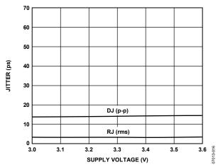
Figure 16. Jitter vs. Supply Voltage
