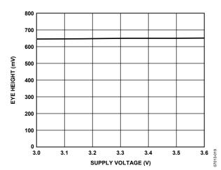
Figure 19. Eye Height vs. Supply Voltage
