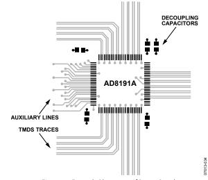
Figure 35. Example Placement of Power Supply Decoupling Capacitors Around the AD8191A
