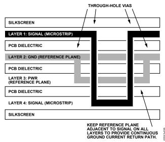
Figure 32. Example Routing of Reference Plane
