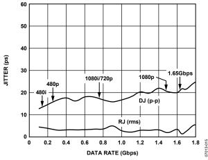
Figure 15. Jitter vs. Data Rate
