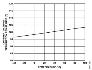
Figure 24. Differential Input Termination Resistance vs. Temperature
