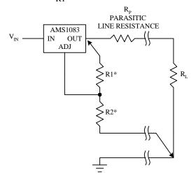
\*CONNECT R1 TO CASE CONNECT R2 TO LOAD
