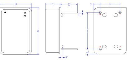
Cover: Kovar Electroless Nickel Plated 1 µinch (25 µm) typical Resistance welded to base
