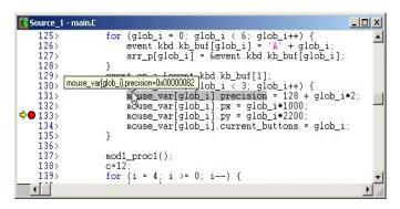
H/W breakpoints and S/W breakpoints (identified by red dots) may be used to stop execution in the critical code sections to allow detailed inspection of the embedded system.
